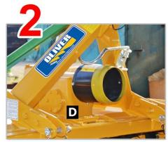
The conical pair is equipped with a gear box **(D)** so to obtain **4** different transmission speeds, depending on the needs of the soil that will be worked.
