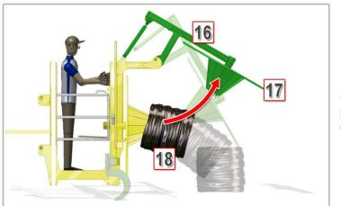
Thanks to the **tilting opening mechanism (16)** of the **hose reel roller (17)**, the unloading of the bundle of the **collected hoses (18)** becomes simple and immediate.
