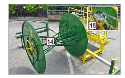
The **coil reel roller (14)** is driven by a **hydraulic motor** powered directly by the tractor's hydraulic system. It is possible to adjust the rotation speed thanks to a **lever flow regulator (15)** placed in the operator's control panel.
