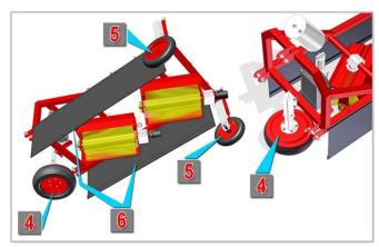
To fix the position of the brushes in height, the machine has a rubberized leveler (4) with variable height.
