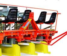
The **frame** is equipped with a **three-point hitch** and the multiple point is raised easily, thanks to the inlets for the **forks of the forklift**.
