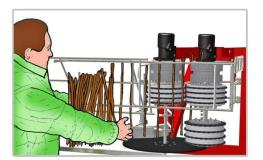
**COLLECTION FACILITATOR KIT**To facilitate the sorting of the plants, a collection facilitator kit is available that allows to reduce the personnel on board. The kit takes the synchronized movement from the hydraulic
