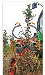
THE CONVEYOR BELT Intercepts the stem of the plant e, varying the speed of the conveyor belt, keeps the olants upright, accompanying them to th
