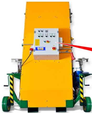
The Soilbagger's mechanical movements are given by three electric engines.
