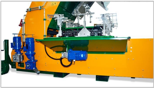
The Soilbagger's mechanical movements are given by three electric engines.
