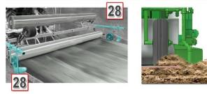
In the first draft of the **nylon film (A)**, the **pivoting arms (28)** are both in the working position.
