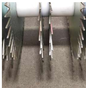
Figure 2 Colibrì, Angled teeth (inter-row spacing 6–7 cm)
